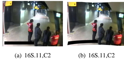
Fig. 8 (a) Presence of the barrel distortion in C2 is more clearly visible towards the left edge of the frame where the vertical structure appears to be bent outwards and (b) distortion corrected frame.
