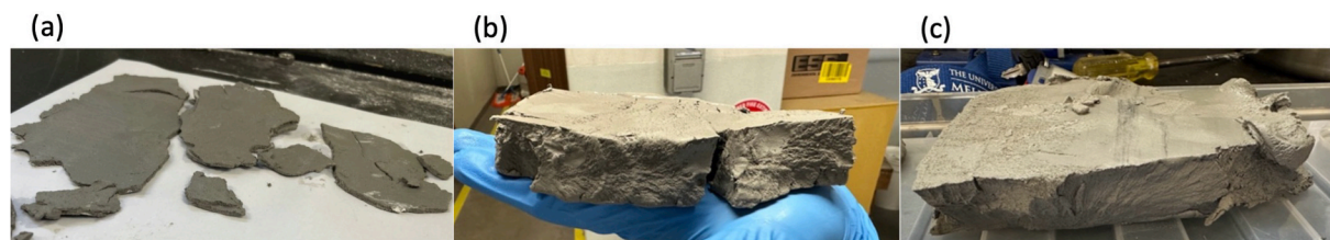
Fig. 7. Filter cakes produced from fully submerged HPDR tests: (a) thin cakes (1 to 3 mm) of flocculated copper, (b) thick cake ( \sim 20 mm) of non-flocculated copper (83.0 wt%) and (c) thick cake ( \sim 20 mm) of flocculated copper (83.1 wt%).
