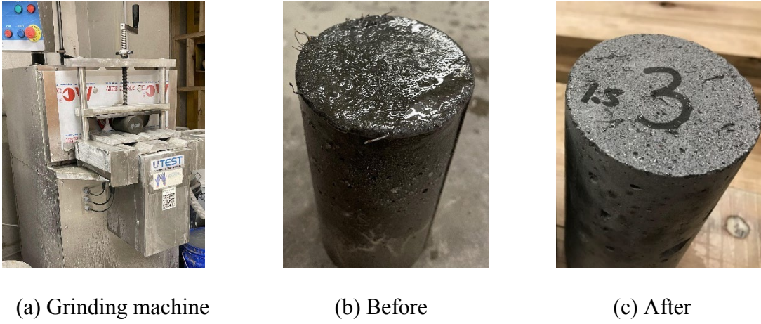
Figure 3 Grinding concrete cylinders
