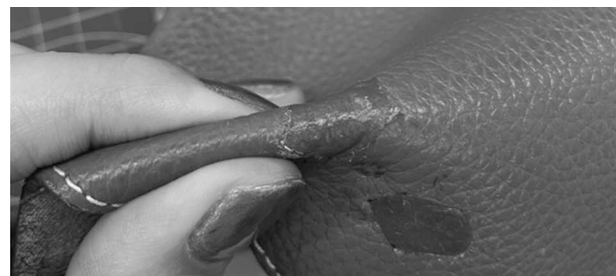
FIGURE 5. 4 gsm Tengu extra light paper fill in 15% Klucel G on a canvas lining during flexibility testing. The fill was able to withstand numerous folding actions without separating.
