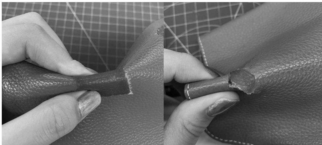
FIGURE 3. Flexibility testing on a large BEVA® 371b fill and a small BEVA® 371b fill. The small fill detached after one fold.
