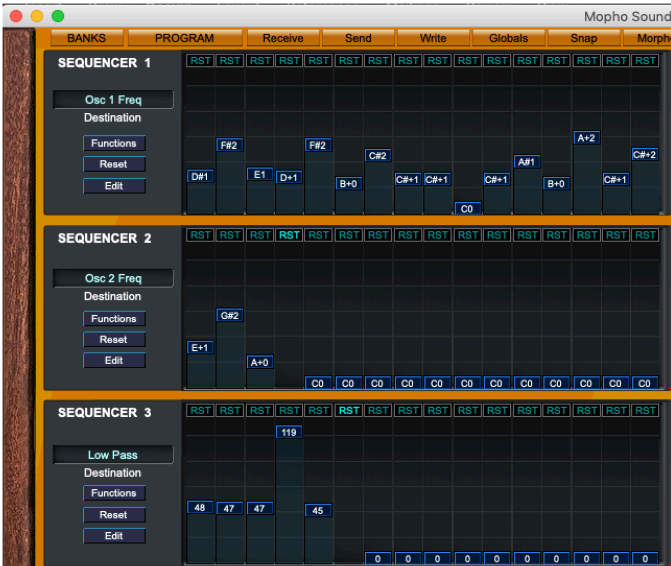
Fig. 2.03 – Three sequences applied polyrhythmically at a ratio of 16:3:5. The highlighted RST on Sequencer 2 and 3 show the point where the sequence is reset.
