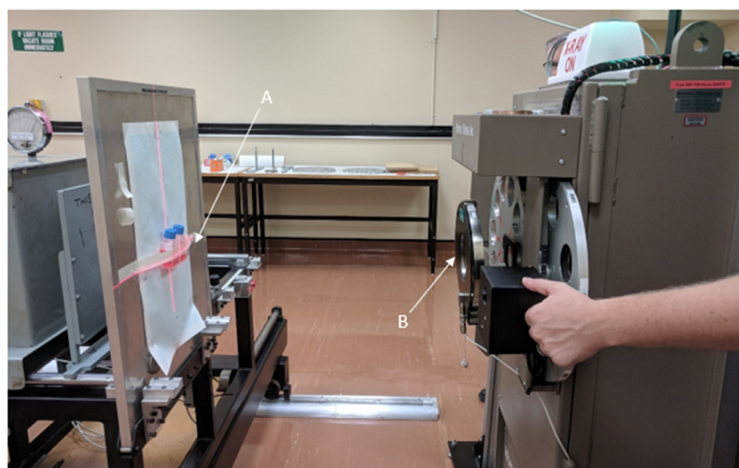
Fig. 3. Image of experimental setup for kilovolt X-ray exposures. Treatment flasks taped vertically to the baseplate (A) of the Model X80 X-Ray Beam irradiator (B). The source-to-surface distance was set at 100 cm to the front of the baseplate.
