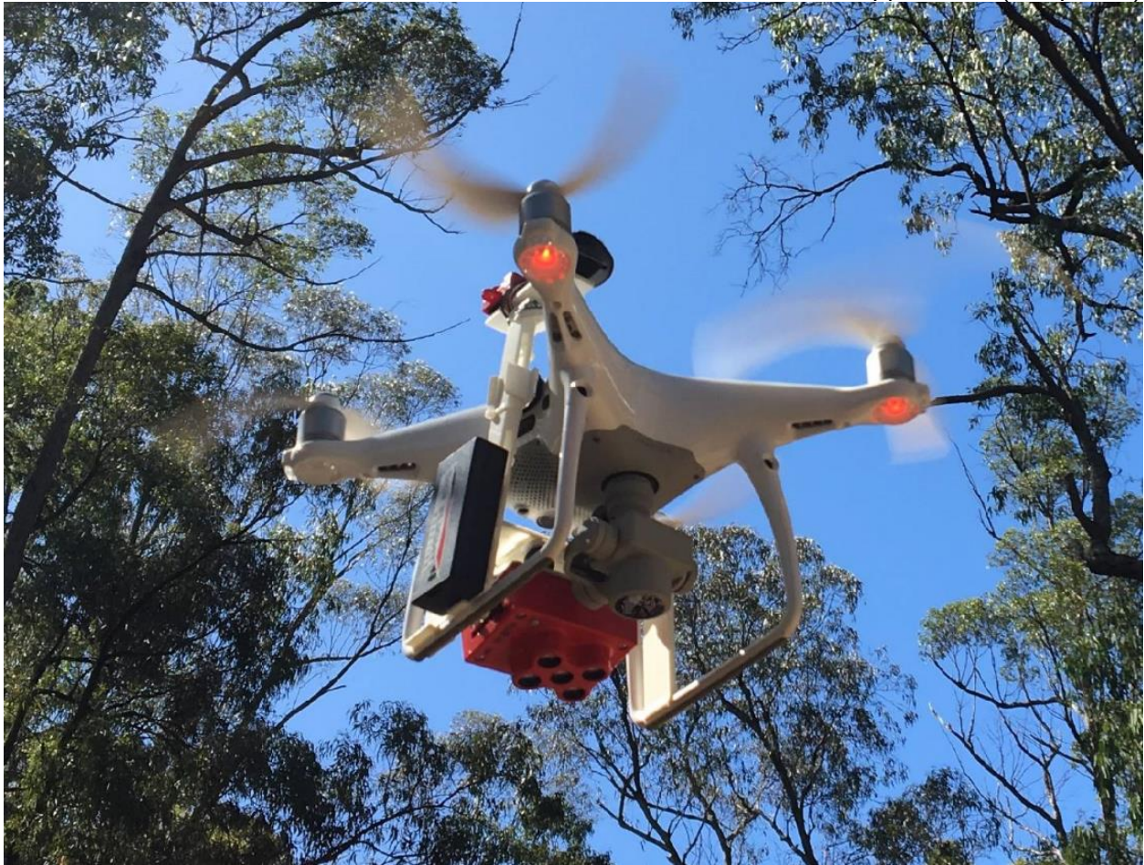
Figure S4. DJI Phantom 4 UAV modified to carry a Micasense RedEdge M multispectral sensor. A 3D printed mount allows to attach the sensor between the landing skids of the UAV. The rod on the left carries the batteries to operate the camera and lifts the radiation sensor and GPS over the propellers for safe operation. This setup allows to capture both multispectral and RGB imagery simultaneously as it leaves the drone's sensor operational. The drone sensor can e.g. be used during operation to check for obstacles or ensure the programmed flight-lines are followed correctly.
