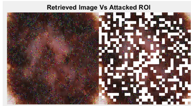
Figure 3.13: Attacked ROI Detected: The sub-blocks with severe attacks has been localised and marked with white boxes
