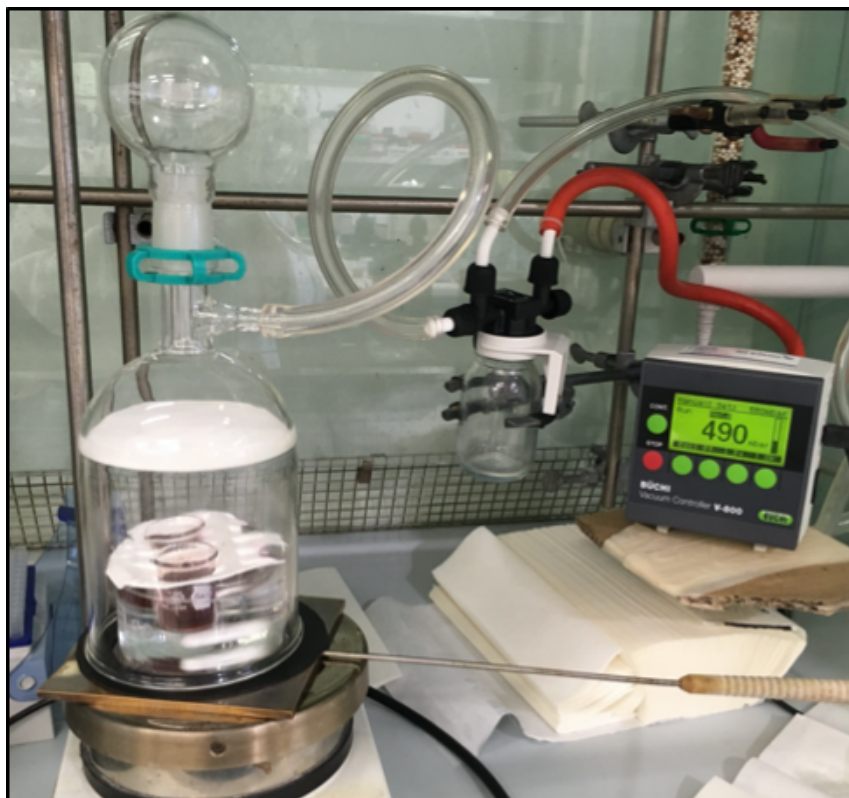
Figure 3.5: Designed set up including a hotplate coupled with a thermocouple and a pressure controller to control the temperature and pressure respectively to evaporate solvent (complete removal)/ non-solvent (up to desired concentration).
