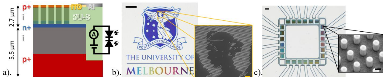
Figure 1: (a) Device schematic (b) Optical microscope image of a fabricated Si NW multi-color image with 50- \mu\text{m} scale bar. Inset shows an SEM image of the Si NWs forming the goddess head, with 5- \mu\text{m} scale bar). (c) Optical microscope and SEM image of a fabricated device. Scale bar: 100- \mu\text{m} . The inset shows a close view of the Si NW array poking out the SU-8 resist and coated with ITO. Scale bar: 0.5- \mu\text{m}
