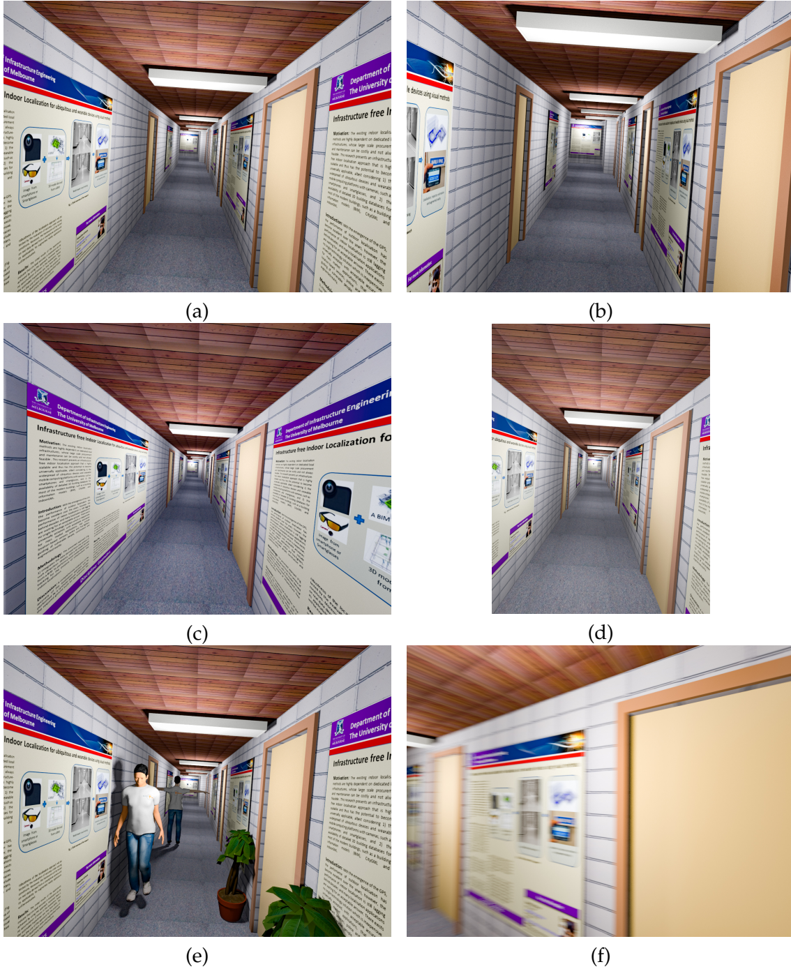
Figure 3.6: An image frame from the set (a) Set 2 - having 90° FoV (b) Set 4 - having 60° FoV (c) Set 5 - having 120° FoV (d) Set 6 - in portrait mode (e) Set 7 - containing walking humans and potted plants as occlusions (f) Set 8 - having motion blur.
