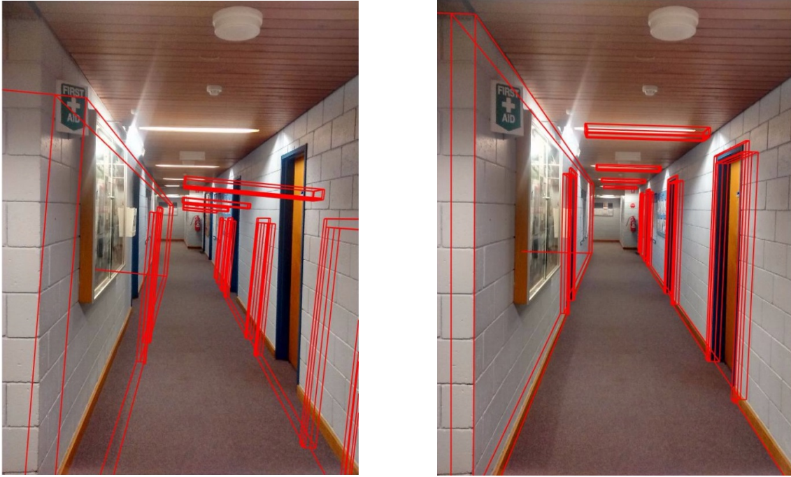
Figure 2.2: An example of 3D model-based visual tracking. The left image shows the projection of initial camera pose and the building edges on the image. The right image shows the overlay of the estimated camera pose after a few iterations.
