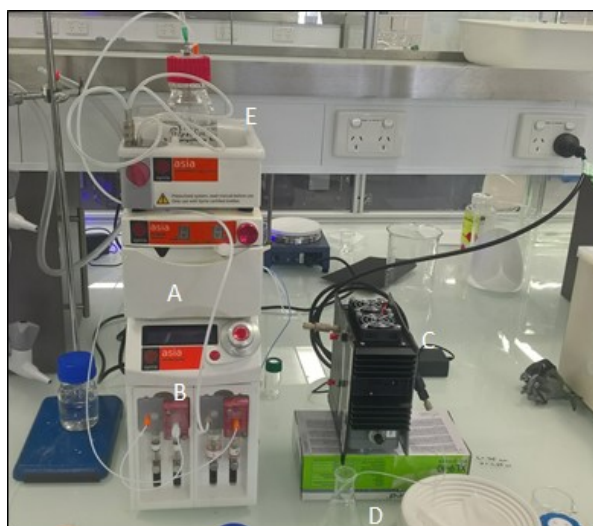
Figure 2.27: Experimental setup for the transfer hydrogenation in flow (A) Sample loop (B) Syringe pump (C) Illuminated photoreactor (D) collection flask (E) Solvent reservoir.
