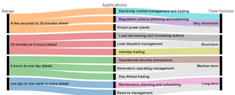
Fig. 1 Wind speed and power forecasting time scale
