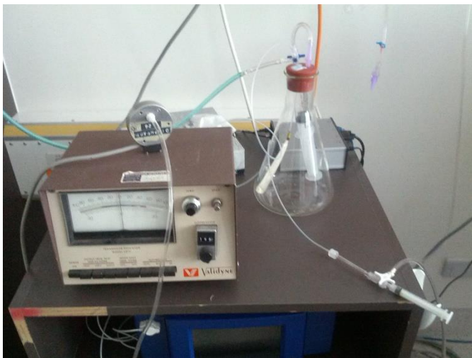
Figure 5.10: Oesophageal Balloon Bedside Calibration
