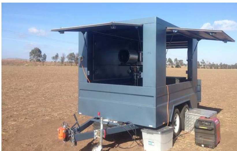
Plate 3 Open path Fourier Transform Infrared Spectroscopy used for measurement of gaseous emissions during field composting (Chapter 4)
