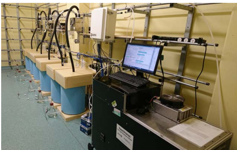
Plate 4 In-vessel composting system with a closed path Fourier Transform Infrared Spectroscopy used for the laboratory scale composting (Chapter 5).
