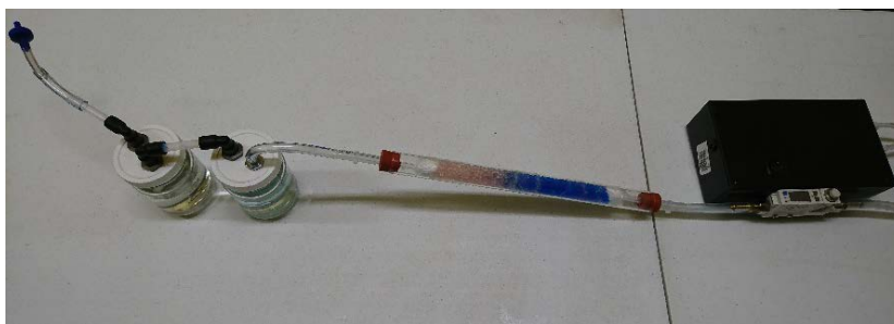
Plate 5 Acid trap used for \text{NH}_3 emission measurements during laboratory scale composting (Chapter 5).
