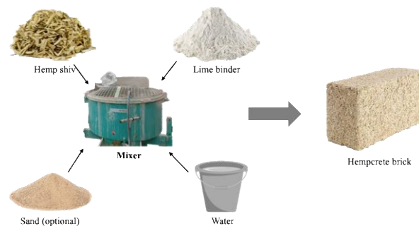
Figure 1: Composition and mixing process of hempcrete materials. (source: Authors)
