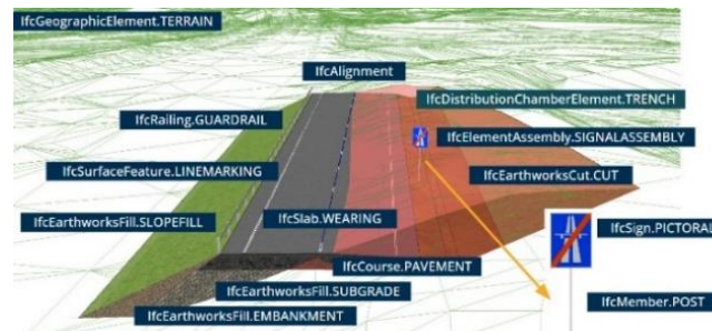
Figure 4: An example of the latest IFC 4.3 attributes for roads, adopted from (Pszczolka, 2022)
