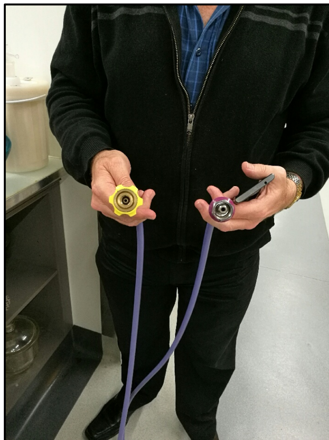
Figure 5.15: A vacuum cable held by Associate Professor Brendan Abrahams. The purple connection is screwed into the anaesthesia machine while, the yellow connection is screwed into a vacuum line fitted on a wall mount in the operating theatre.
