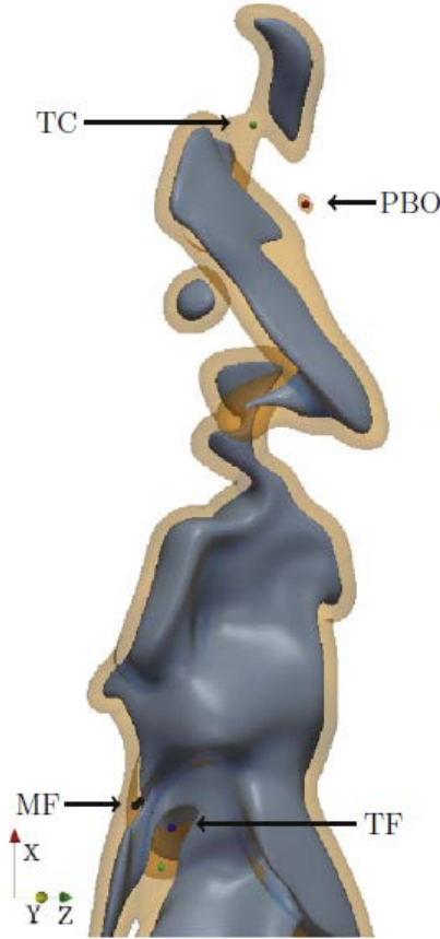
Figure 7: A snapshot of the flame with the identified annihilation events using the critical points in the progress variable field. The two iso-surfaces represent the progress variable range used in the searching algorithm.
