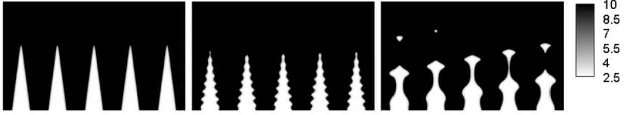
Figure 4 : Non-dimensional temperature fields at St = 1 (left column), St = 0.1 (middle column) and St = 0.025 (right column) of the perturbed flame at several instants during a forcing cycle. The Strouhal number is defined here as St = fL_{ref}/c_{ref} where L_{ref} is half of the inlet width and c_{ref} is the speed of sound at the inlet.
