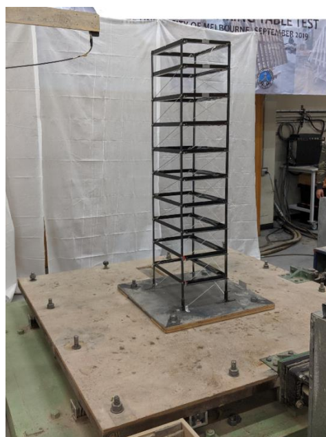
Figure 4-24 Experimental set-up of conventional steel building on the shaking table
