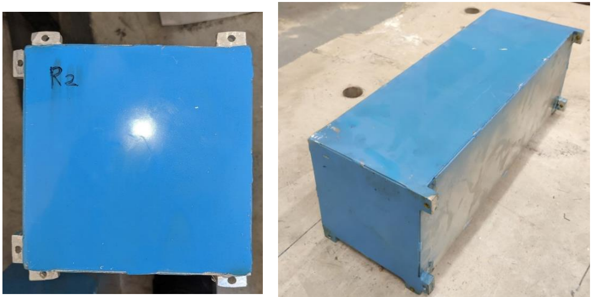
Figure 4-3 Protrusions at the module face providing connectivity between modules
