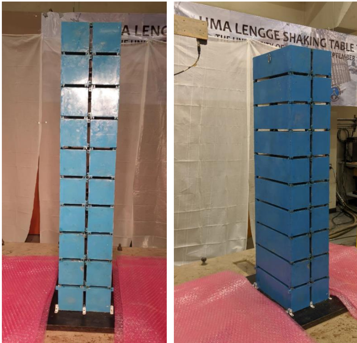
Figure 4-14 Experimental set-up of the modular building on the shaking table
