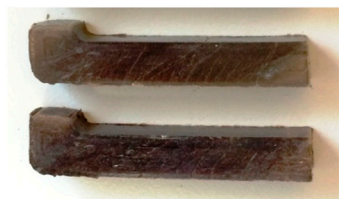
Figure 4. Typical equal channel angular pressing (ECAP) consolidated samples (left) and their optical images of microstructures showing regions with cracks (black arrows) in (a) HW/PEI, (b) HW/PEI/TA, (c) HW/PEI:A, (d) HW/PEI/TA:A, and shear bands (between dashed lines) in (e) HW/PEI:M, (f) HW/PEI/TA:M, (g) HW/PEI:(A + M), (h) HW/PEI/TA:(A + M). The white arrows mark the general particle orientations. The pressing direction is horizontal to the right.
