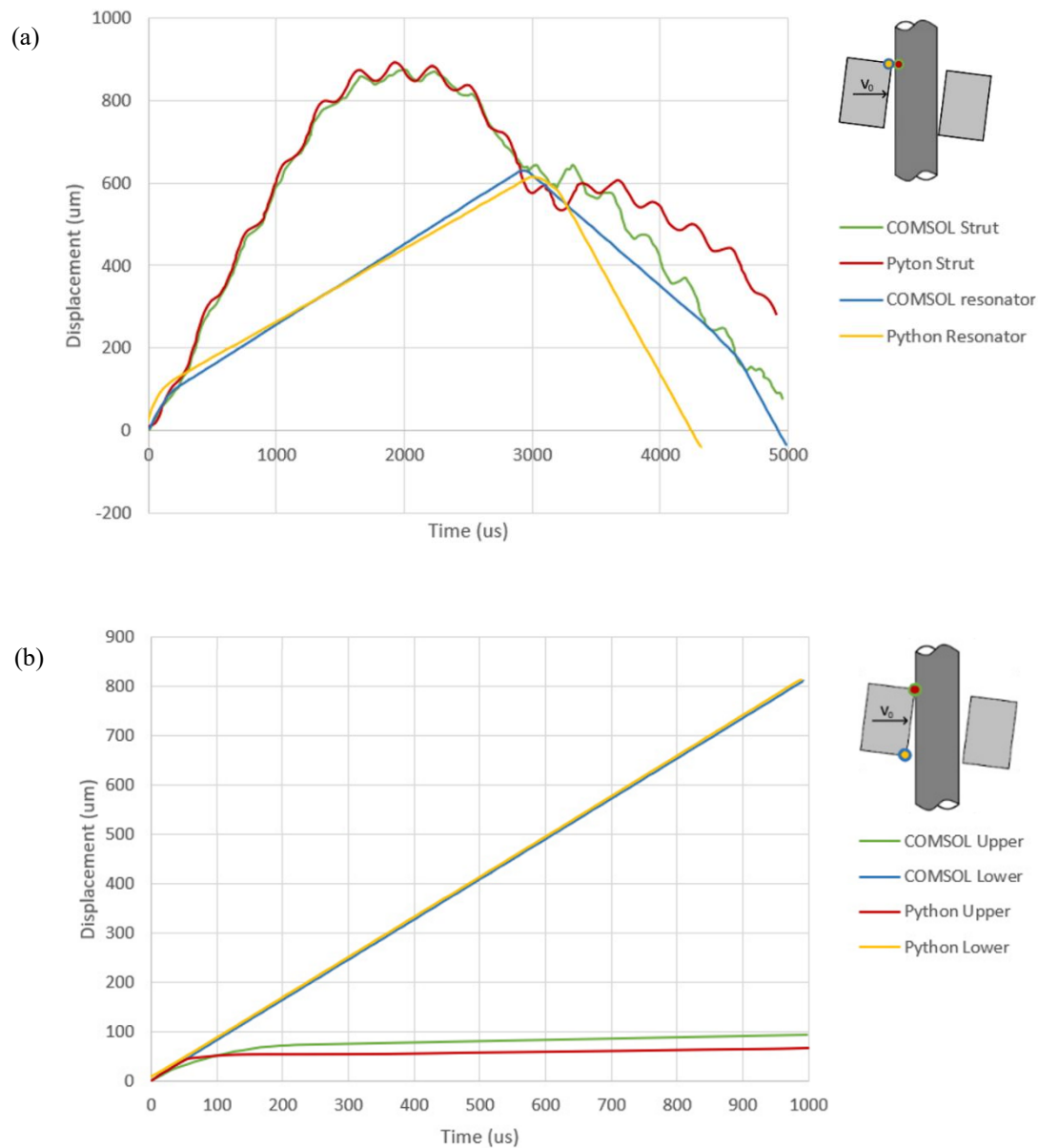
Figure 4.12 Transient displacement of contact points for resonator and structure after a single impact. The structure was initially at rest, and the resonator had initial velocity, V_0 = 0.83 m/s. In (a), displacements at the point of contact on both strut and resonator are compared over the course of 0.05 s. In (b), the rotation response of the resonator is assessed by tracking two points on the resonator over the course of 0.01 s the resonator was given an initial velocity ( V_0 ) of 0.83 m/s and the impact occurs in the first 50 \mu s
