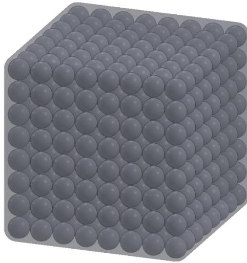
Figure 2.11 Illustration of three-dimensional lattice of locally resonant silicone rubber coated lead spheres presented in Liu et al. [82]
