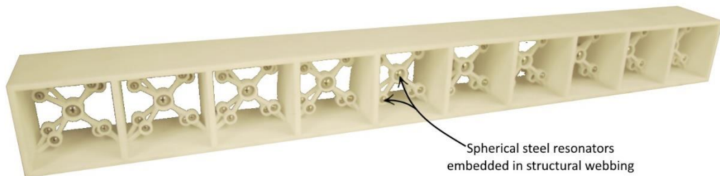
Figure 2.16 3-D printed prototype of an inertial amplification beam structure with structurally integrated resonators [116]
