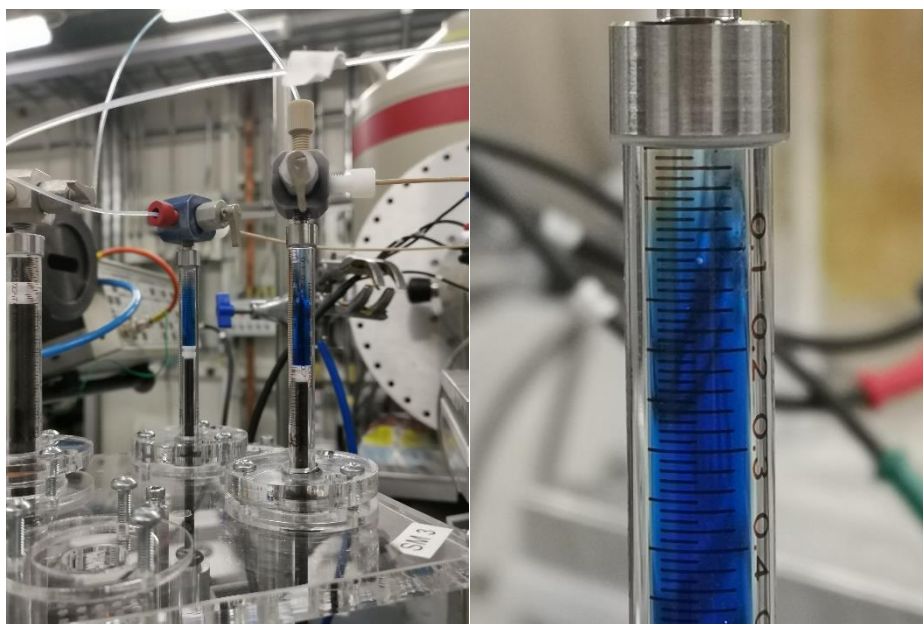
Figure 3 Solutions of a copper(II) complex together with the redox mediator DCIP (dichlorophenolindophenol) following multiple passes of 100 \mu\text{L} of the XAS-SEC cell at reducing potentials. The oxidised form of DCIP is an intense blue and the reduced form colourless. A closeup view of the receiver syringe is shown.
