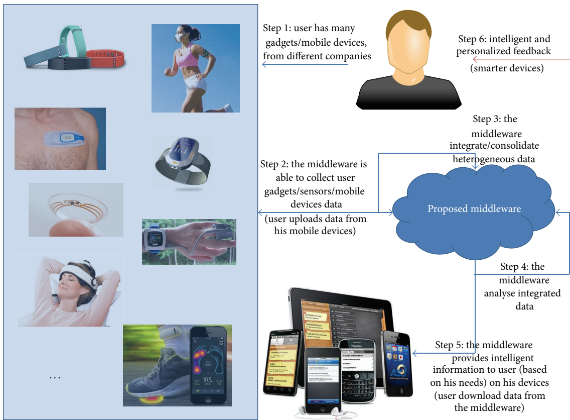
FIGURE 2: A conceptual intelligent middleware: Device Nimbus. This model is based on the integration of mobile sensor data for Smarter Services focused specifically on fitness sensors/device.
