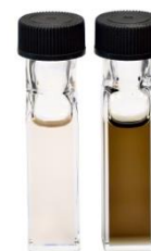
Figure 7. Distinct colour changes occur upon addition of fluoride to the cyclophanes. This example shows the change with 0.5mM of 6 in DMSO in the absence of F^- (left) and with the addition of F^- (right).
