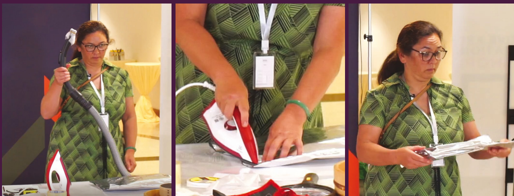
Figure 219: Vacuum hose to extract the air out (left), Iron to seal the Marvelseal foil bag (centre), Final vacuum sealed package with the painting inside, oxygen scavengers and oxygen indicators (right)
