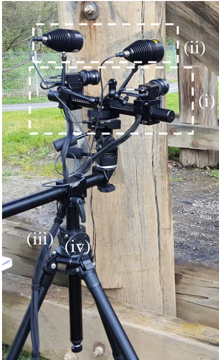
Figure 3.1: Detail of 3D optical measurement system components: (i) right and left cameras; (ii) camera lights; (iii) cable connecting the cameras to data acquisition box; and (iv) tripod
