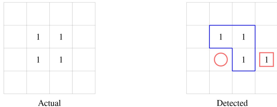
Fig 11. A toy example depicting an actual and detected event. The actual and detected event pixels are labeled as 1 with the intersection or true positives marked with a blue outline. The false positive and false negative pixels are marked with a red square and circle respectively. The Jaccard index for the detected event is 0.6.
