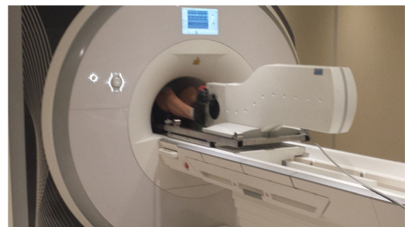
Fig. 3 Lode BV supine cycle ergometer during in-scanner supine exercise cardiac magnetic resonance. The Lode BV supine cycle ergometer allows in-scanner exercise, up to maximal exercise intensity, during CMR scanning, as demonstrated by La Gerche et al. [29]. The ergometer attaches firmly to the CMR scanner bed by screw attachments and is safe to use in CMR scanners up to 3 T. The patients' feet attach into the stirrups and strap securely in place. Resistance can be altered manually in 1-watt intervals. This ergometer is the most utilised modality in Ex-CMR research studies
