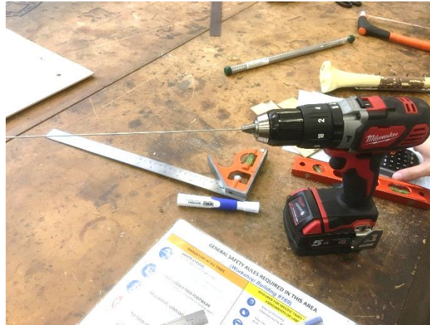
Figure 3.3 Wires affixed to drill driver (Milwaukee, Wisconsin, USA).
