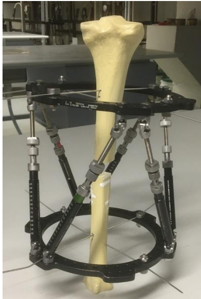
Figure 2.7 Taylor spatial frame (TSF) mounted on a surrogate human tibia (shinbone)
