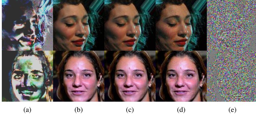
Figure 1: Adversarial perturbations generated by AdvFlow take the structure of the original image into account, resulting in less detectable adversaries compared to \mathcal{N} ATTACK [33] (see Section 4.1). The classifier is a VGG19 [50] trained to detect smiles in CelebA [36] faces. (a) AdvFlow magnified difference (b) AdvFlow adversarial example (c) clean image (d) \mathcal{N} ATTACK adversarial example (e) \mathcal{N} ATTACK magnified difference.
