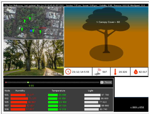
Fig. 8. Real-time interactive geovisualization of multivariate data of each sensor node: Visualization includes spatial information of sensor nodes, selection of sensor node using marker, panoramic view of selected sensor node with context information, visualization of microclimate parameters and canopy coverage, bar plots of all sensor nodes data and time slider to choose real-time data or time range for historical data. Brightness of panoramic view changes according to luminosity data, while temperature and humidity are visualized using color gradient and blur change in tree background respectively.
