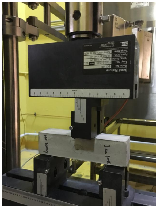
Fig. 2. The three-point flexural bending strength test with the testing machine and a prism paste sample while testing.
