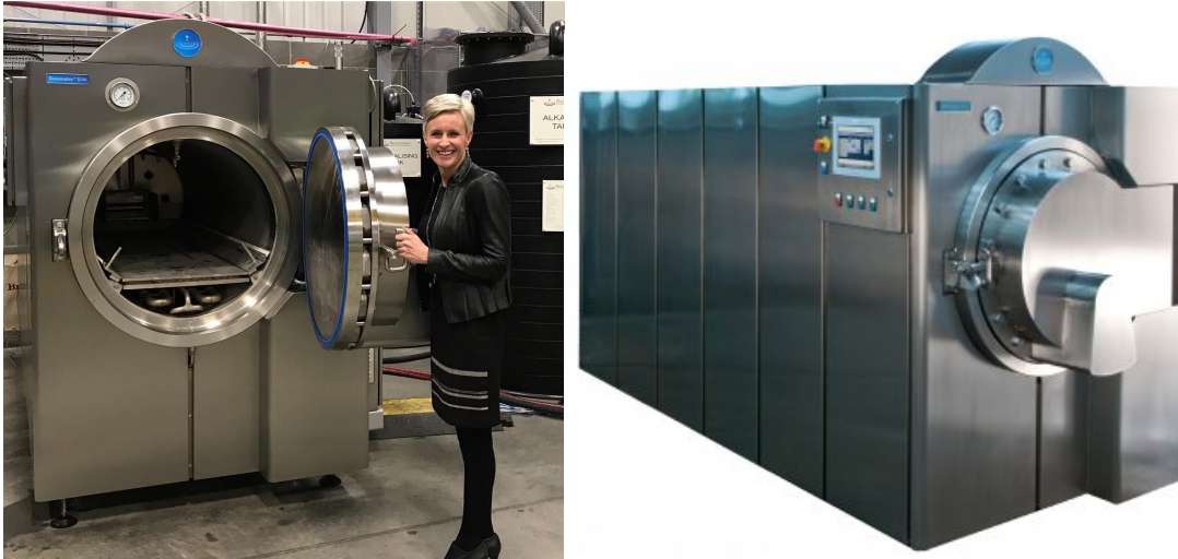
Figure 1. Examples of alkaline hydrolysis retorts manufactured by Resomation. (Images sourced from Resomation)
