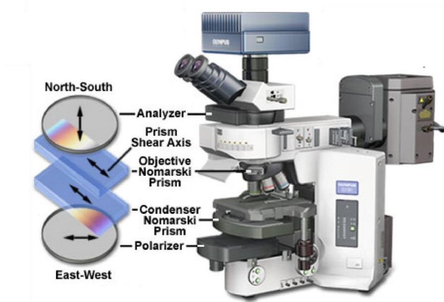
Figure 3. A DIC microscope. Polarised light enters a Nomarski prism and reorientates to produce a wavefront. Subsequently, the wavefront passes through a condensing lens to form parallel components and that probed onto the sample. After that, the
