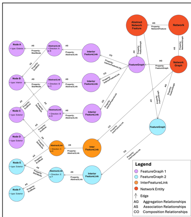
Figure 6. NetworkGraph sample including InteriorFeatureLink and InterFeatureLink
