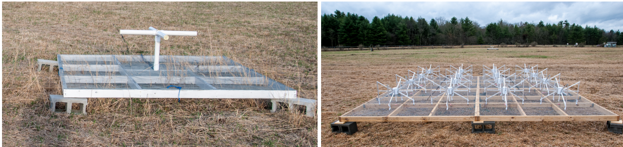
Figure 2. Reference antenna on 2\text{ m} \times 2\text{ m} ground screen (left) (see Section 2.3) and MWA antenna tile on 5\text{ m} \times 5\text{ m} ground screen (right) (see Section 4) deployed at the National Radio Astronomy Observatory–Green Bank.
