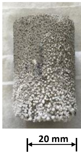
501 Fig. 6. The white reaction products precipitated on the sample surface clogging the surface pores after 56-day 502 immersion period (The picture was taken after the sample was taken out from the acid solution and dried 503 under ambient condition for upto 3 hours).
