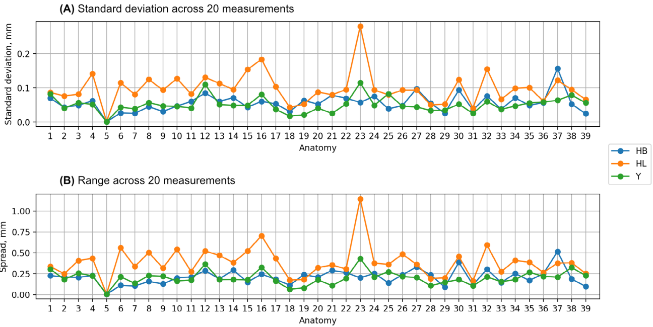
FIGURE 3 Accuracy of the automated pipeline measured by (A) the standard deviation across 20 runs and (B) the range between the highest and lowest measurements.
