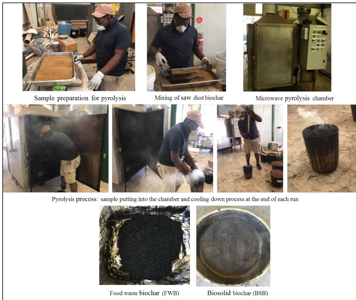
Figure 4.1 C: Steps of preparation of biochar using a microwave pyrolysis setting.
