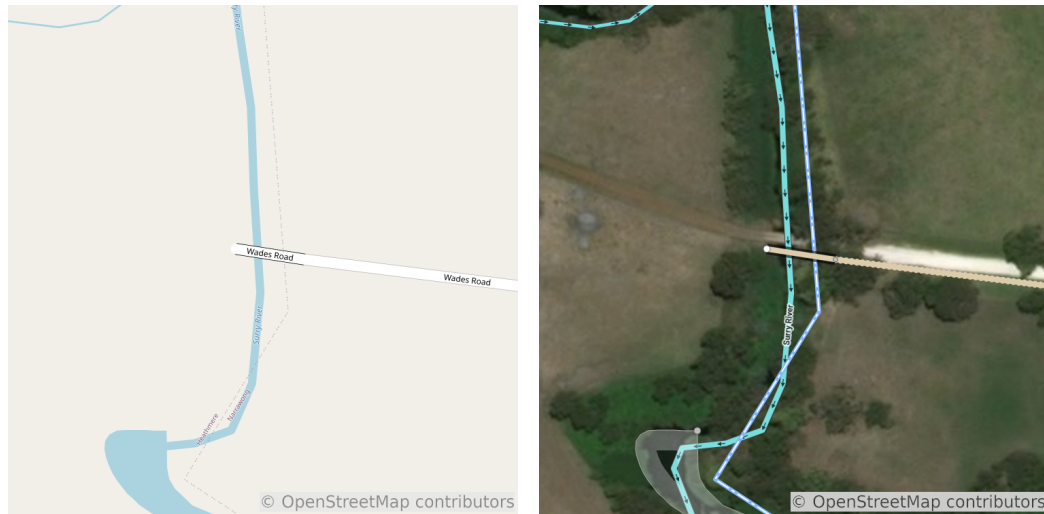
FIGURE 1.1: An example of a map, showing a dead-end bridge that is disconnected on one side (left) and the satellite imagery of the same area that shows that there exists a road or a path that is connected to the bridge, but is not mapped (right).
