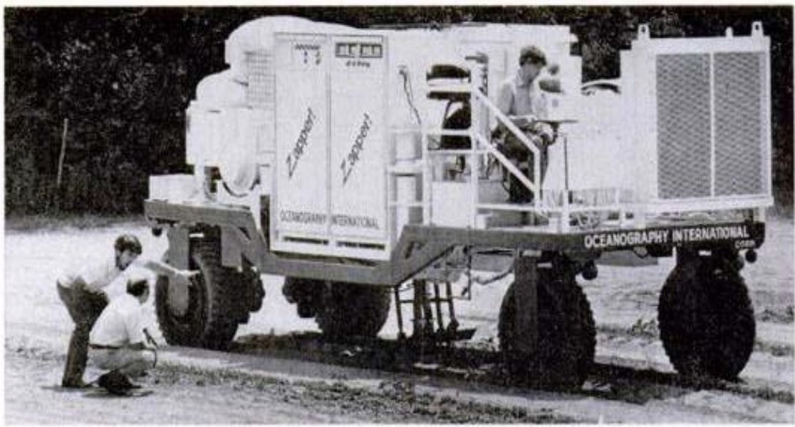
Figure 2.5: The Zapper III (60 kW; microwave weed killer) developed by Phytox Corporation to zap weeds and soil treatment under field conditions.
