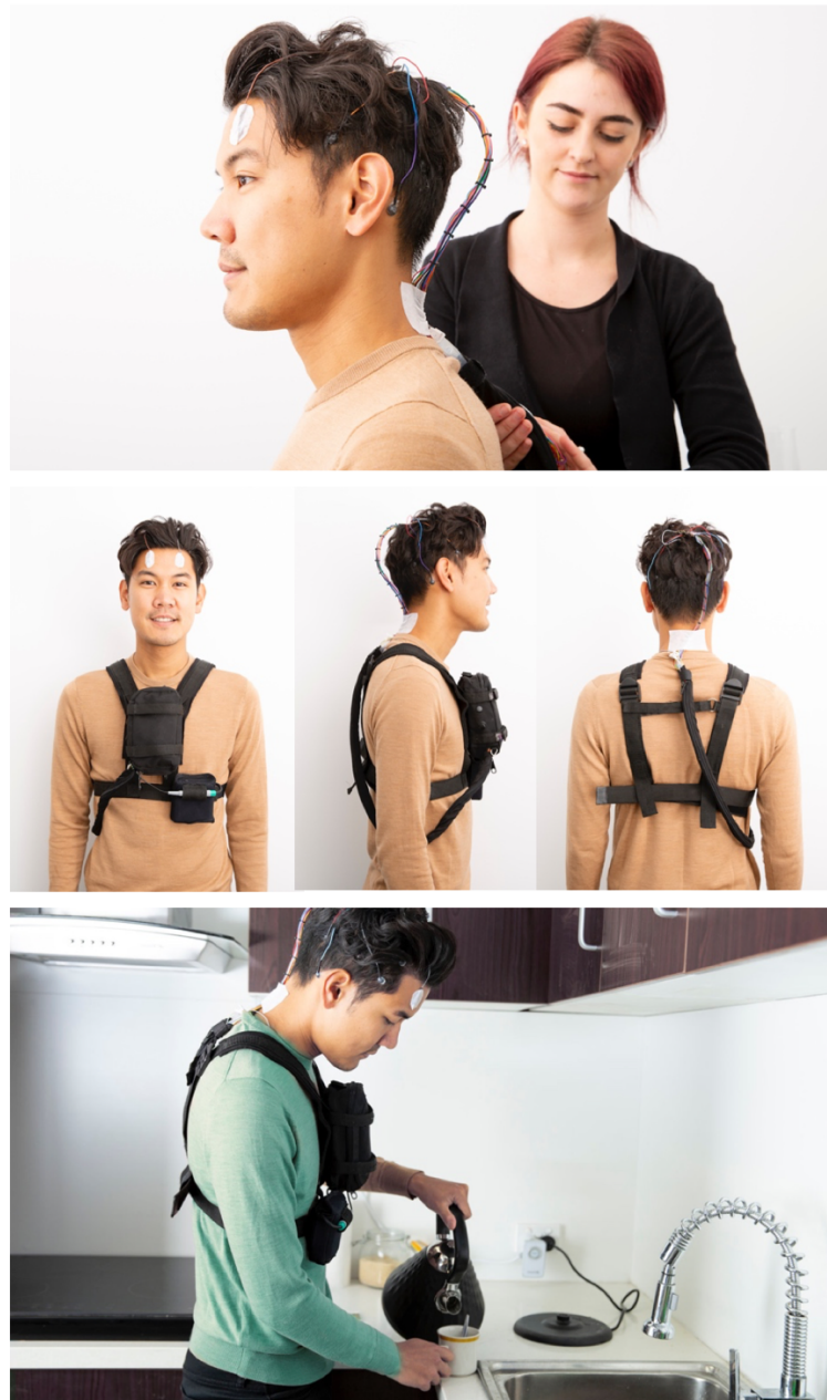
Figure 6. Example images of the portable EEG-ECG recording system in practice. The system is first attached by a trained neurophysiologist at Seer Medical (top). Electrodes are glued to the scalp. Wires are connected, gathered, and brought down the back of the participant's head. These are held in place with enough slack for the participant to move their head and neck without pulling at the wires. These wires all connected to the recording system, transmitter, and battery pack worn by the participant (middle). Participants are then sent home to continue about their daily lives (bottom). They are free to move about and complete daily tasks with little restriction from the equipment (From https://www.seermedical.com ).
