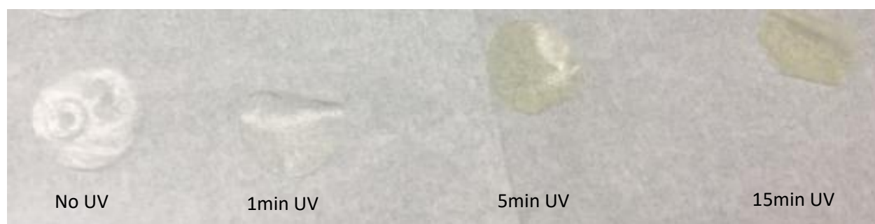
Figure S2. Coloration of PVDF-HFP based membrane upon longer UV-irradiation.
