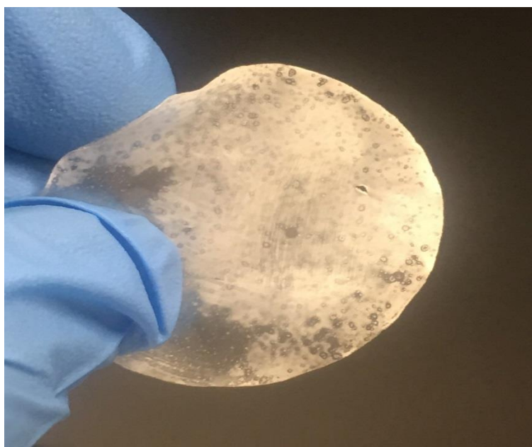
Figure S4. Photographic image of a non-cross-linked PIM (40 wt% D2EHPA, 10 wt% NPOE and 50 wt% CTA) after the second extraction/back-extraction cycle.
