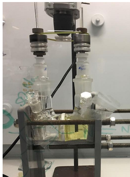
Figure 5. (a) Schematic presentation of a transport cell and a generic PIM facilitated ion-exchange transport mechanism in the case of a monovalent target cation ( A^+ ). N^- , counter anion; X^+L^- , ion-exchange extractant (carrier); X^+R^- , stripping reagent. (b) Photographic image of the transport cell set up in the laboratory.
