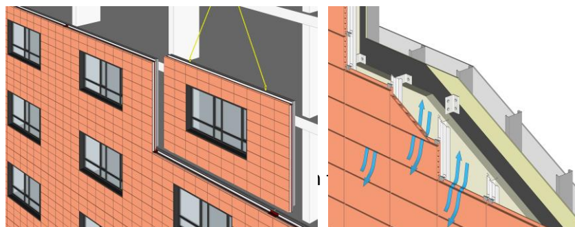
Figure 2.5. Unitised rain screen façade system [12]
