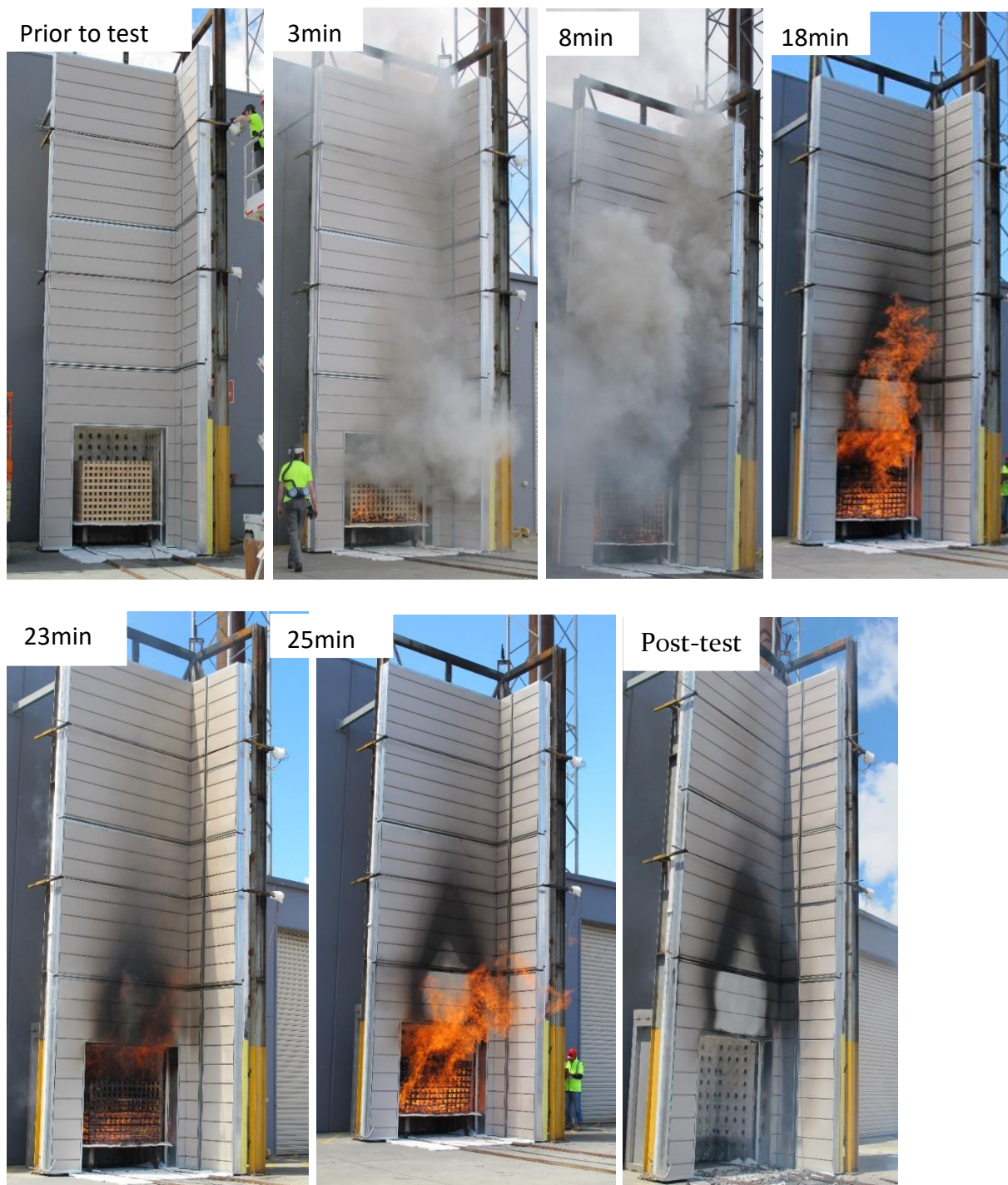
Figure 5.13. CSR full-façade fire test in accordance with AS 5113 and BS 8414-2 test method
