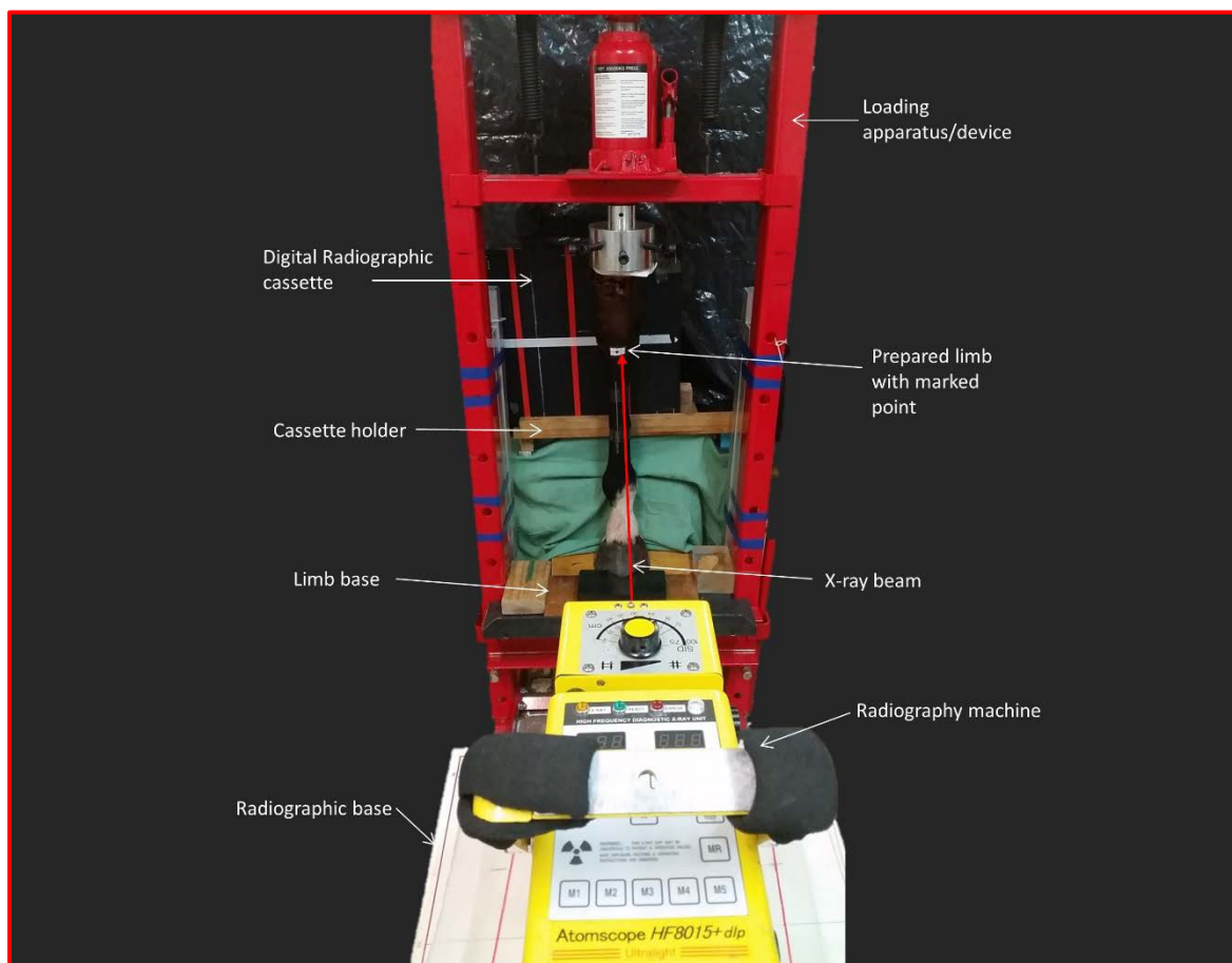
Figure 4. 2: Radiographing a right tarsus of a thoroughbred. The cadaveric articulated distal hind limb was fixed in the limb base. The radiographic machine was placed on the radiographic plate. The central x-ray beam was directed perpendicular to the talus as indicated by putting landmark on the limb.
