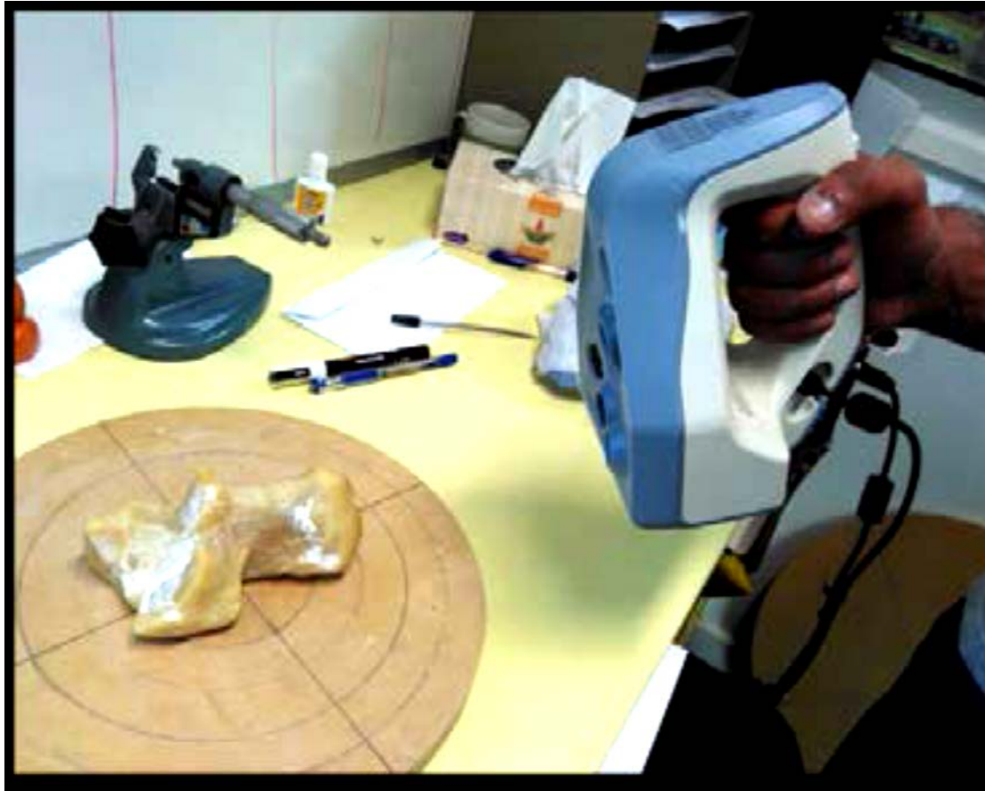
Figure 13.1: Scanning of right calcaneal bone of thoroughbred horse using ARTEC 3D scanner.
