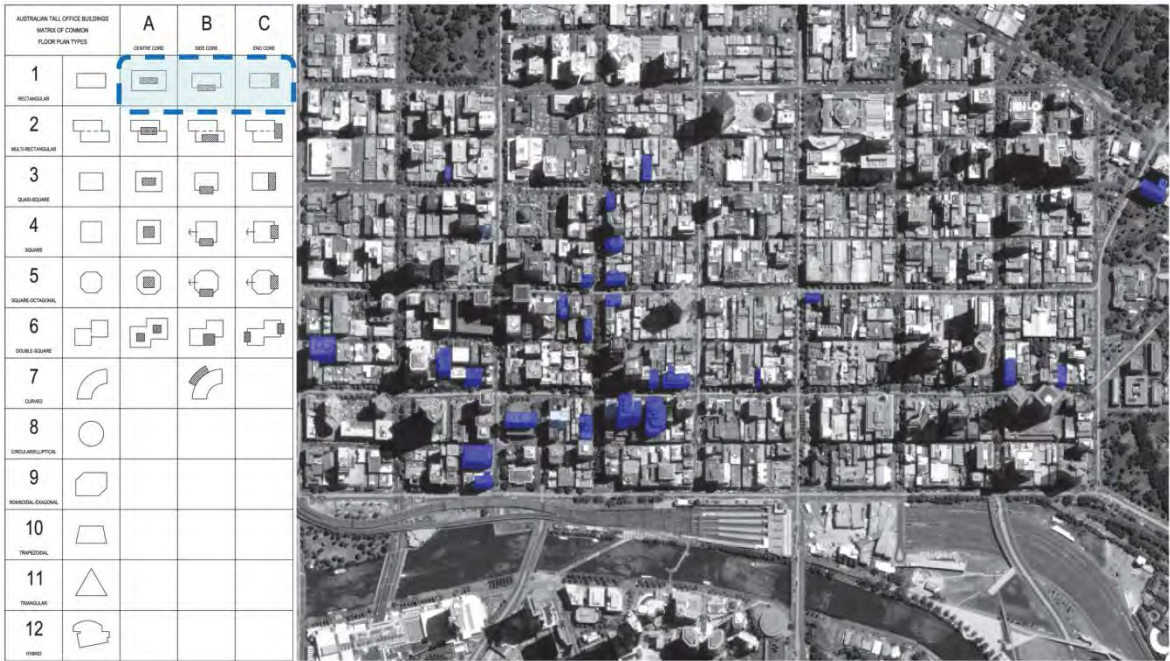
Figure 1.3 Tall office buildings in Melbourne CBD with rectangular floor plan type
