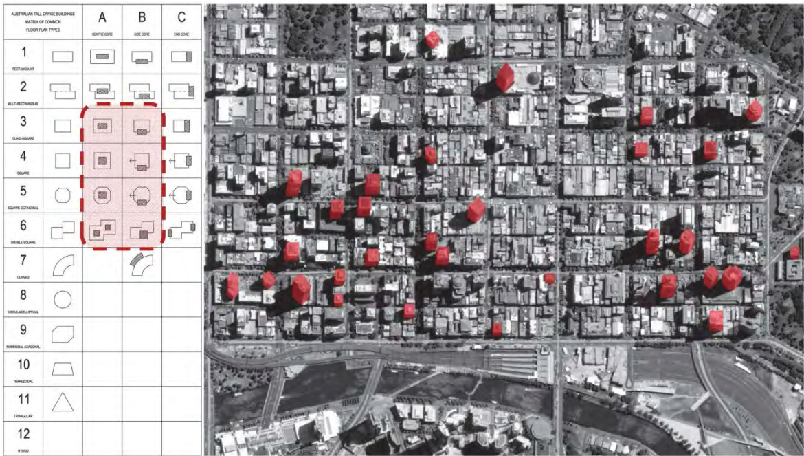
Figure 1.4 Tall office buildings in Melbourne CBD with square or quasi-square floor plan type
