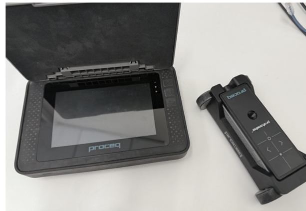
Figure 7. A profometer 600 unit.
