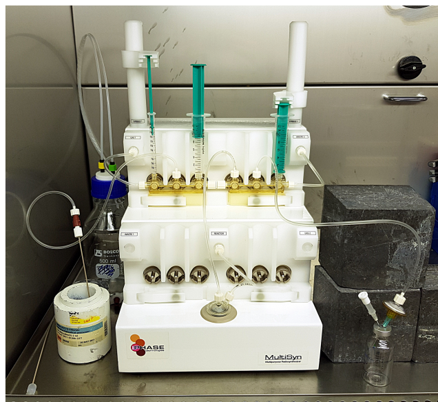
FIGURE 3 Picture of iPHASE MultiSyn set-up for automated radiosynthesis of [ 177 Lu]Lu-PSMA-617 according to Figure 4 and Table 1
