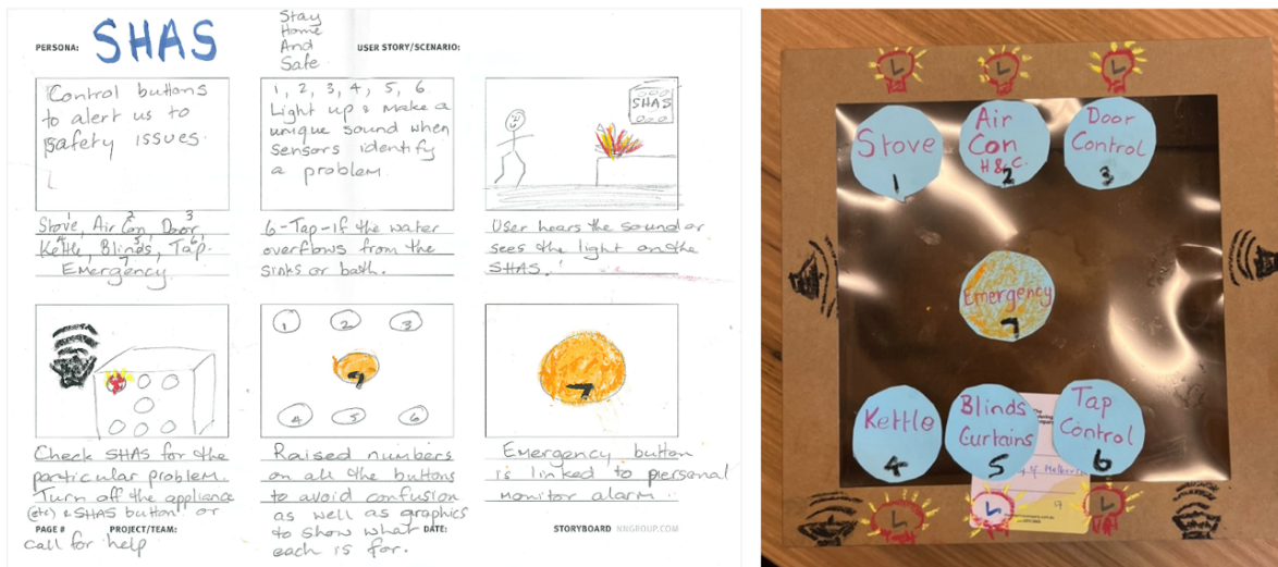
Figure 6: Participants' design of a home control system called SHAS. It allows users to control home appliances through a box-shaped panel, receive alerts when potential safety concerns are detected, and use the system to call emergency services.
